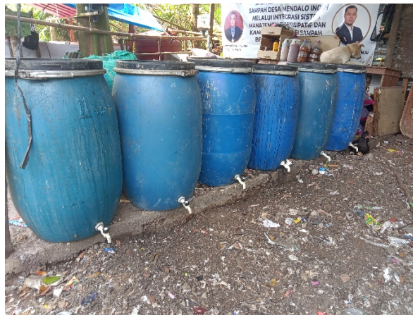
Figure 3. 120 L Composting Drum
